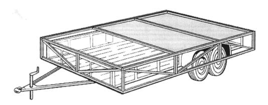
Attachment of skirt frame and sheet plywood.
